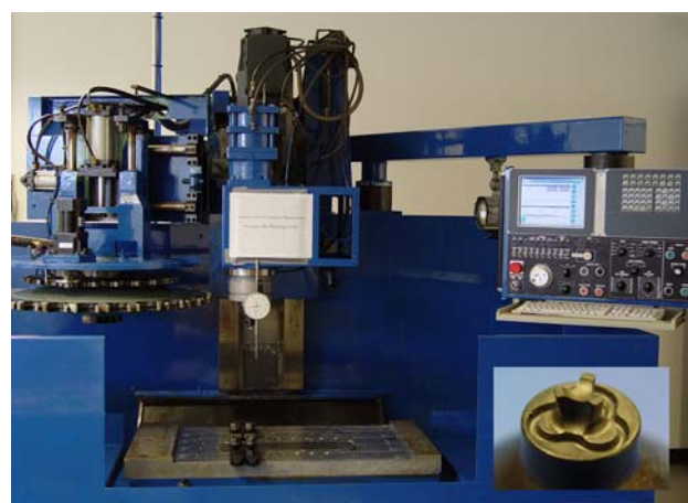
Fig. 1 CNC-controlled friction stir welding with 2D welding capability. Inset: Tool used for friction stir lap welding of aluminum sheets
