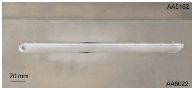
Fig. 5 Friction stir lap welded AA 6022-5152 sheet
